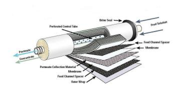
Water is forced to circulate under high pressure through porosities on membranes which has 5 angstrom diameter of pore. While water molecules and some inorganic molecules can pass through these porosities during this process most substances in water cannot pass through these porosities and it is exhausted as concentrated water.
