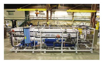
Reverse osmosis process is the removal of dissolved solids from the water by pressurizing the water through a semi-permeable membrane. Reverse osmosis is used purification for well water, river water, lake water and seawater which has high salinity.
