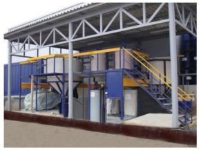
Package type of industrial waste water treatment plant (I-WWTP) can contain one of or all of physical, chemical, biological and tertiary treatment methods depending on raw wastewater quality & quantity.
