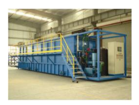
When used with domestic wastewater, MBR processes could produce effluent of high quality enough to be discharged to coastal, surface or brackish waterways or to be reclaimed for urban irrigation. Other advantages of AKTIFPAK-MBRs over conventional processes include small footprint, easy retrofit and upgrade of old wastewater treatment plants.
