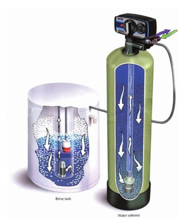
Softening is the removal of hardness in water caused by calcium and magnesium ions using cationic resin.
